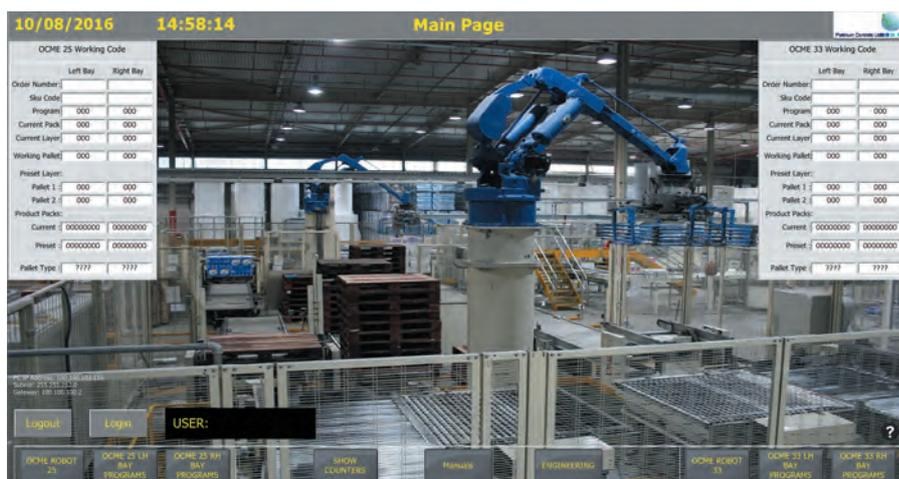
Platinum recommended the Progea Movicon system (available in the UK through Products4Automation). The system controls the robot's programs from a database of many different pallet-filling patterns, which are chosen according to the size and shape of the multipacks being palletised and/or to meet individual customer preferences.
